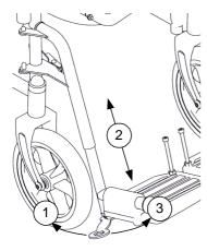
For optimum comfort it is important to attain the correct leg position. The footrests have been designed so that they can be extended into a number of fixed positions. To do this, release the bolt using the spanner (see diagram) and turning clockwise (1). Then adjust the footplate to lengthen or shorten the legrest (2). Finally, tighten the bolt by using the spanner and turning anticlockwise (3).
