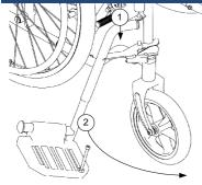
To remove the leg rest, press the chrome lever on the leg rest whilst swinging the leg rest out. This will now allow the leg rest to be lifted up and removed. To attach the leg rest, place the leg rest on the two receiver posts on the wheelchair frame (1). Then swing the leg rest inwards until it locks in position (2).
