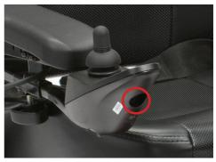
NOTE: The Titan18LC powerchair comes with interchangeable shrouds, allowing you to customize your powerchair to your liking. All models come with the red shrouds installed, and a spare set of blue shrouds included in the box. The shrouds can be interchanged by hand, or using a small pry tool. Be sure not to scratch the painted shrouds while using the pry tool.
