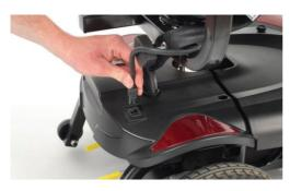
8. Plug the cable from the joystick remote in to the port at the back of the powerchair base.
